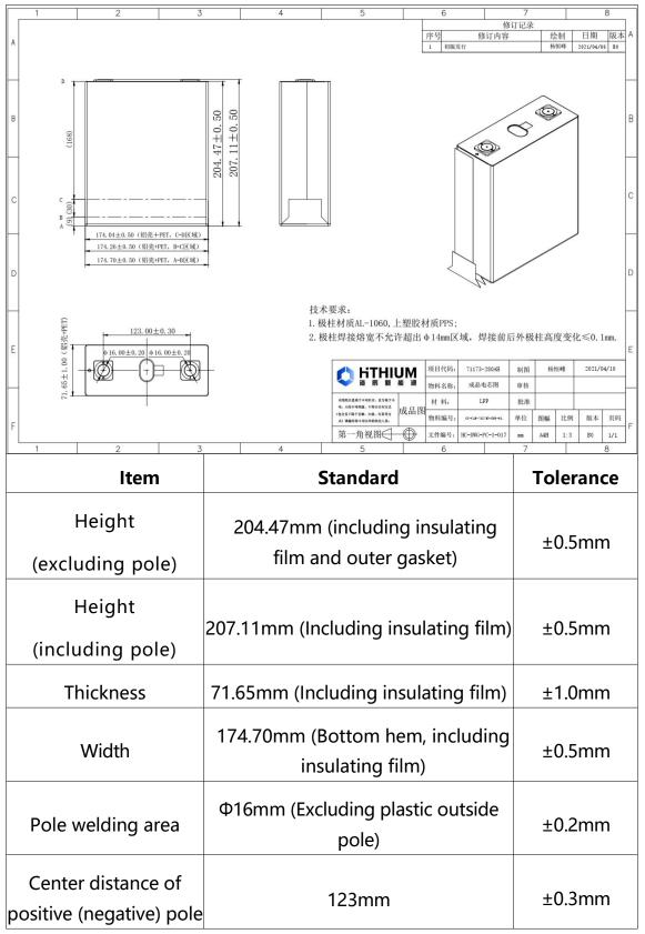
Note: the thickness is measured under the condition that the large surface pressure is  $3000 \pm 200$ N
